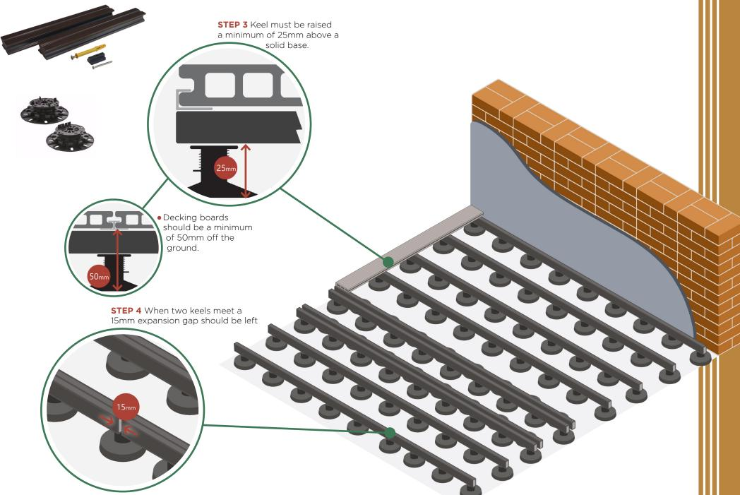
**STEP 5** Determine how you are going to lay out your decking. Lay a suitable geotextile membrane & position the pedestals and keels.
